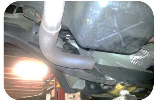
Figure 6 Exhaust after cutting
