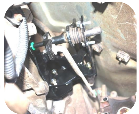
Figure 9 Transfer Case Linkage Installed
