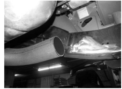
Figure 5 Exhaust after cutting
