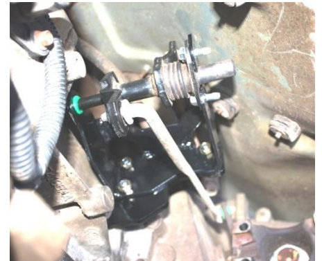
Figure 7 Transfer Case Linkage Installed
