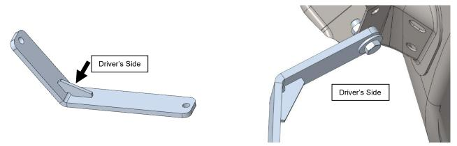
8. Install the passenger's side support arm into the forward-most hole on the engine mount bracket on the frame. Use a 1/2" bolt, washer and nut. Do not tighten the hardware at this time.
