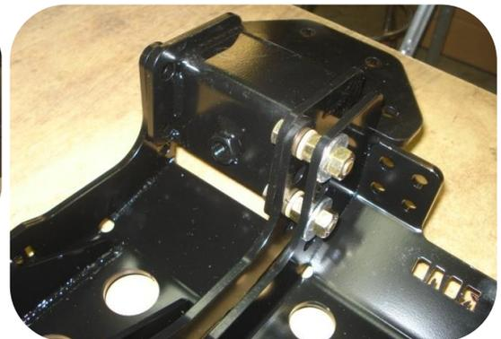
5. Place the belly skid against the nuts on the back of the subframe, install washers and nuts hand tight. Match the holes in the skid to the holes in the subframe. **Example:** If your subframe bolts are in the upper set of holes, put your belly skid in the upper set of holes.
