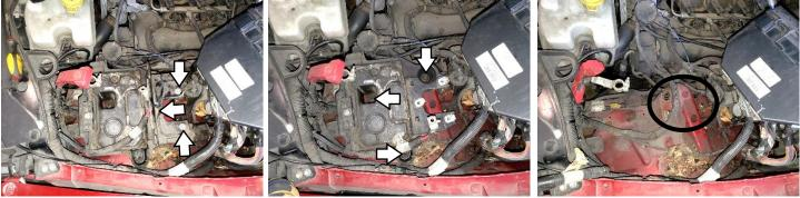
9. This will give you access to the nuts securing the strut assembly to the body. Do not loosen at this time.
