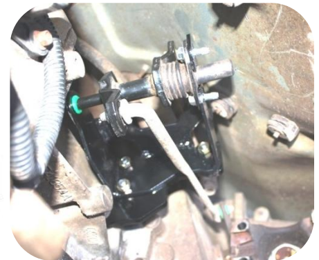
Figure 9 Transfer Case Linkage Installed
