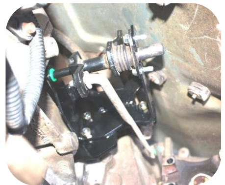
Figure 9 Transfer Case Linkage Installed
