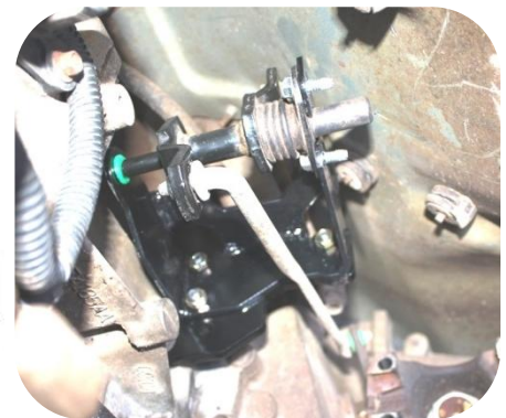
Figure 9 Transfer Case Linkage Installed
