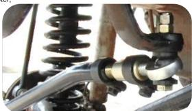
upward angle on the drag link where it meets the rod end. Meaning the drag link angles only up and forward from the rod end, not down then back up. The rod end should be pivoted so that the drag link can never drop below this 5-degree angle.
