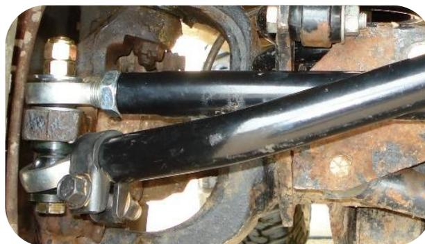
**For 33-36" tire diameter** (measured): adjust your tie rod until the front measurement is 1/8" less than your rear measurement. Adjustment can be done by removing only the driver's side bolt and you can turn the whole tie rod if needed to adjust both sides equally.
